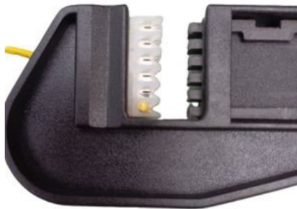
Terminal block held in tool, yellow wire already
